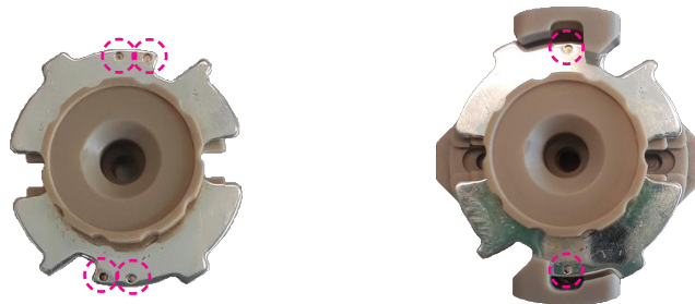
Figure 3: The upper fluid cell has four dots (left) used to lock the cell in position. When the cell is locked in place only one dot on each side will be visible (right).
