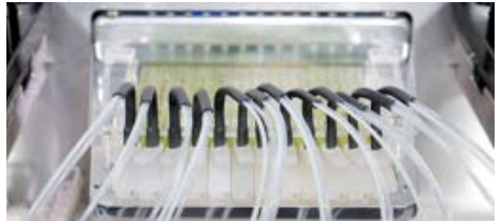
12 ingredient inputs with tubing that can be used with any virtually any container
