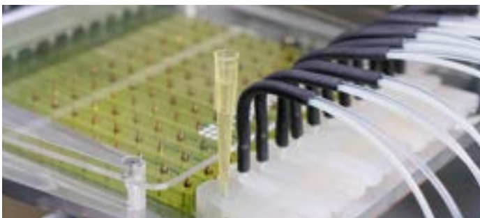
direct pipette tip dispenses reduce dead volumes of only 100 \mu L
