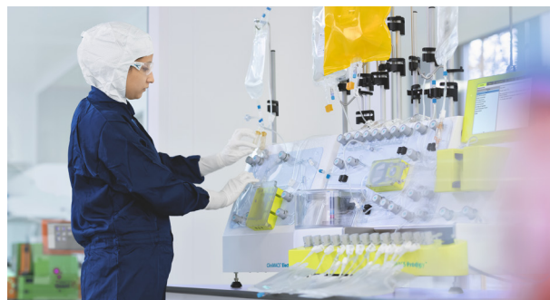
Figure 3: Complex cell manufacturing processes, including electroporation, are performed in the closed system of the CliniMACS Prodigy.
