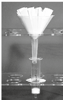
Figure 2 Correct use of the NucleoBond® Folded Filter, NucleoBond® Column placed in a Plastic Washer (reusable)
