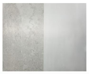
Processing by the pickling passivation machine - before (left) and after (right)
