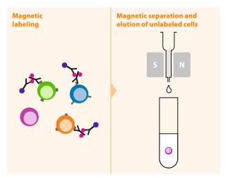
Figure 3: Untouched isolation with MACS Technology. Non-target cells are magnetically labeled. During separation, the unlabeled target cells are collected in the flow-through fraction, while non-target cells are retained within the column.
