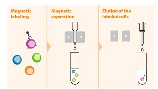
**Figure 2: Positive selection with MACS Technology.** Target cells are magnetically labeled. During separation, the magnetically labeled cells are retained within the column, while unlabeled cells flow through. After a washing step, the column is removed from the magnetic field of the separator and target cells are eluted from the column.
