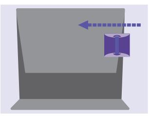
2. Check that the ejection block in the gap of the magnet is attached before placing the MACS Column into the magnetic field of the MidiMACS Separator. Do not remove ejection block of the MidiMACS Separator.
